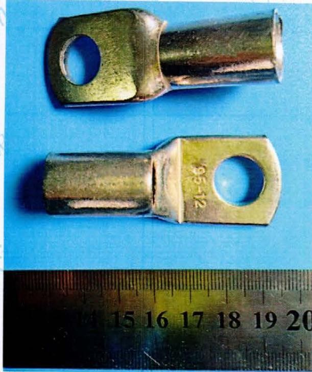
A photograph showing two metal components, likely terminals or connectors, placed above a metric ruler. The components have a cylindrical body with a flared base and a central hole. The ruler is marked in millimeters from 15 to 20.  |
